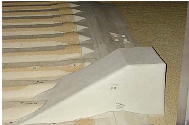
Figure 3.2-1-2. ET forward bipod ramp (foam).
